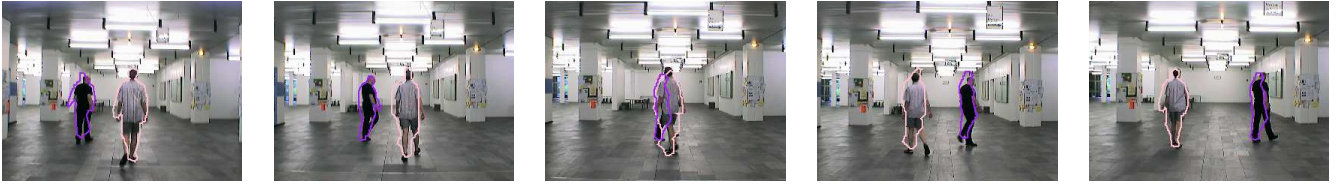
Fig. 8. Outtake of the first experiment. The two persons are crossing their paths. The time gap between two images is one second. The matched contour based on the particle with the maximum a posterior weight are overlaid in pink and purple. The robot was moving at a speed of 60 cm/s during this experiment
