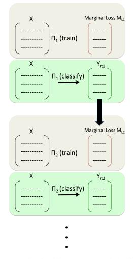
Fig. 1: Schematic of training a sequence of classifiers for regret reduction of contextual sequence optimization to multiclass, cost-sensitive, classification. Each slot has a dedicated classifier which is responsible for predicting the action with the maximum marginal benefit for that slot.
