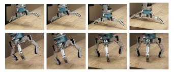
Fig. 11: Compliant fingers landing/placement experiments from different hand pre-shapes
