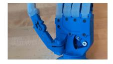
Fig. 9. Revolute joint at the base of the thumb.
