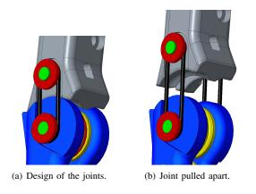
Fig. 2. Rotational sliding joint.
