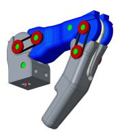
Fig. 4. Finger in fully closed configuration.
