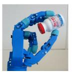
Fig. 16. Precision grasp using the spherical configuration.
