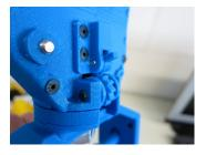
Fig. 11. Locking mechanism with ratchet and pawl.
