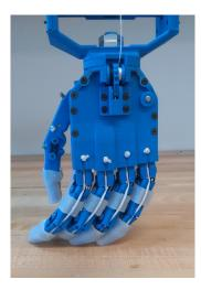
Fig. 5. Lateral deformation of the hand.
