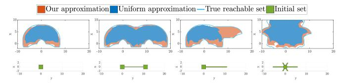
Fig. 2: Left-to-right: Set of initial conditions and the resulting reachable set for the unit cube, dumbbell, lollipop, and hedgehog scenarios. We compare the reachable sets of uniform sampling, our algorithm, and the ground truth. The visualizations show that uniform sampling initial states performs poorly when the set of initial states has an uneven distribution of volume.
