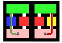
(a) Static mobile-manipulation domain images presented to AMT users for annotation. Positive (green) and negative (red) labels were applied to the images so that AMT users could infer the constraint reflected in the robot's behavior.
