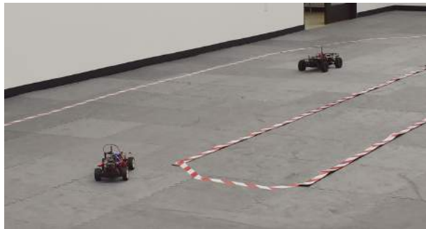
(a) Indoor experiments using RC car experimental platform. Motion capture system is used for odometry information of both cars.
